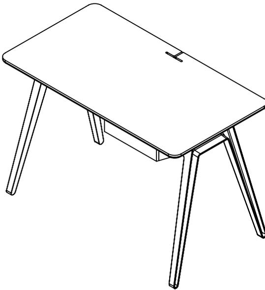
b) If the desk is rocking, slightly loosen the three bolts connecting the legs to the desk body. If this is done while the desk is in its natural upright position, it will allow the legs to settle into the best possible position for the floor upon which it rests. After finding the best position, tighten the bolts firmly.
