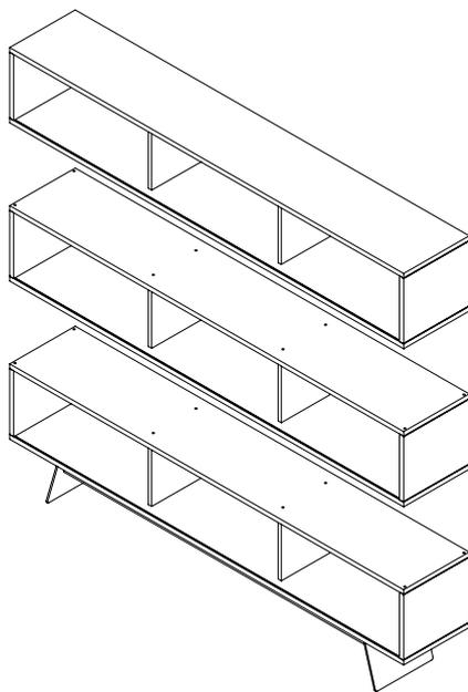
b) Place the second module on top of the first module, and align the holes. Insert an M8 conic bolt into the pre-drilled holes and into the matching metal inserts and tighten firmly with a 5mm Allen Key, but do not overtighten.
