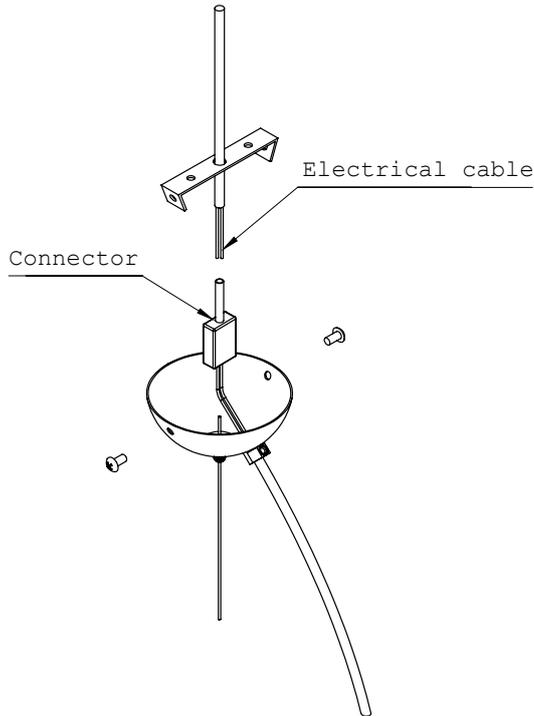
b. While holding the ceiling rose against the ceiling, align the holes on the sides of the ceiling rose with the holes in the sides of the anchor plate.
